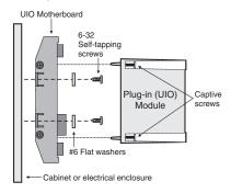
SIGA-MIO: mount the UIOxR motherboard inside a suitable GE Security enclosure with screws and washers provided. Plug the module into any available position on the motherboard and secure the module to the motherboard with the captive screws. Wiring connections are made to the terminals on the motherboard (see wiring diagram). UIOxR motherboard terminals are suited for #12 to #18 AWG (2.5 mm² to 0.75 mm²) wire size.
